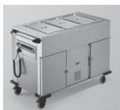
Food transport trolleys made of stainless steel. Worktop with ridge edge, deep-drawn heated wells, welded-in, wet and dry heating with drain. Dry heating results in considerable energy savings. Wells for GN containers 1/1 up to 200 mm. Cupboard, doors double-walled, insulated. Dimensions per compartment: 330 x 570 x 438 mm, 1 heated compartment on left, 1 refrigerated compartment on right.
