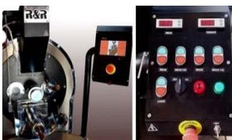
R&R coffee roasters control boards have 2 options; manual control and touch screen PLC control. Manual control comes with separate start stop buttons of each motor, burner switch and emergency stop buttons. 2 thermostat with indicators for drum and exhaust temperature.
