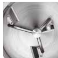
Mixing device with three arms Mescolatore a tre braccia
