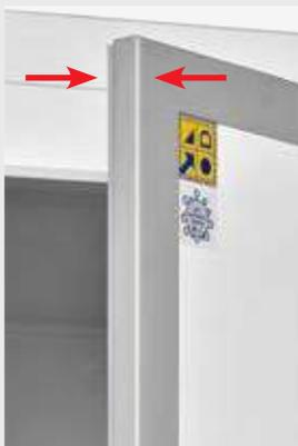
The **half recessed door** has a footprint into the corridor of only 4 cm. Advantages of this type of door are: less space occupied, less volume to be cooled at the same capacity, an air tight seal created by a wider magnetic door gasket.
